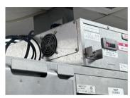
EVO Heads- Each side of the EVO line has a little fan with a cover. Wipe the fan area a few times a week to prevent dust and build up. This saves the life of the fan and prevents the EVO overheating.
